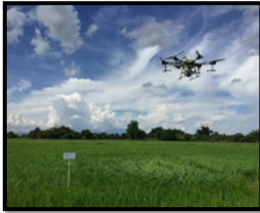
Fig. 2 Unmanned Aerial Vehicle (UAV) used as an aerial fungicide sprayer to control rice blast disease at the vegetative stage.
